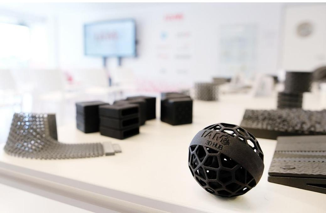
3D printers offer product developers the ability to print objects in **one piece**, without having to assemble any parts and offering a wide range of product **customization**, the **recycling** of materials and the absence of **waste**.
