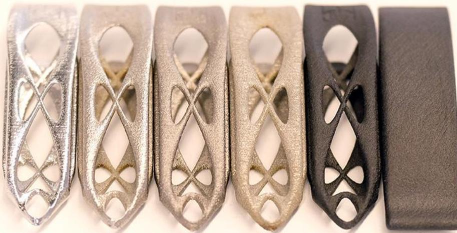
Example of an **optimized piece** with different **additive manufacturing** and **post-processing technologies**.
